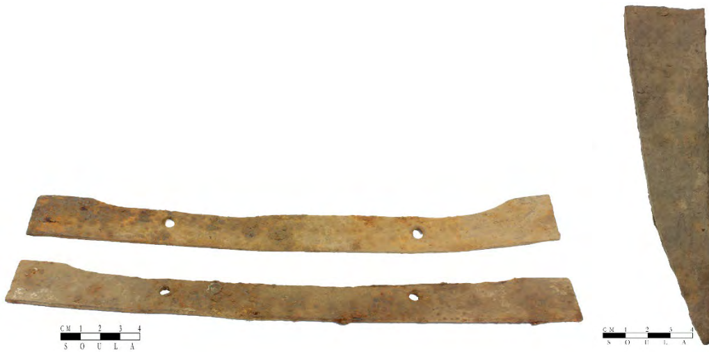
Figure 99. A sample of the Ah Heng II tools. Left: handmade log peeler/planers ( Specimen 2019.07-0037 , Specimen 2019.07-0036 ). Right: pick tip ( Specimen 2019.07-0040 ).
