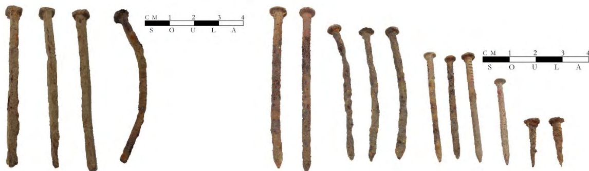
Figure 20. A sample of the nail assemblage recovered from the site. Left: cut nails ( specimens 2018.10-0051 and specimen 2018.10-0088) and wire nails and tacks ( specimen 2018.10-0023, specimen 2018.10-0022, specimen 2018.10-0119, specimen 2018.10-0090, specimen 2018.10-0120, and specimen 2018.10-0101).
